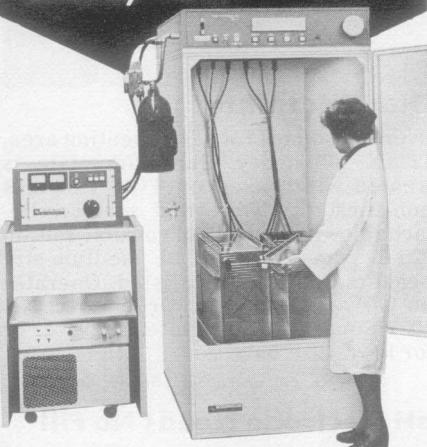
**SAVANT'S HIGH VOLTAGE ELECTROPHORESIS ENCLOSURE WITH TWO LUCITE TANKS.**
